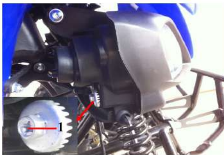
1. Headlight beam adjusting bolt
